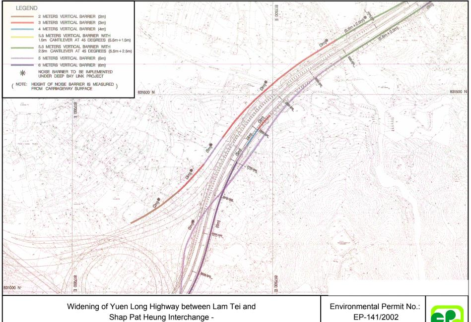
Location of Noise Barriers to be Constructed before Operation of Project
